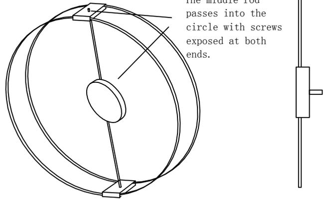
6. Install the upper and lower parts of the intermediate rod.
