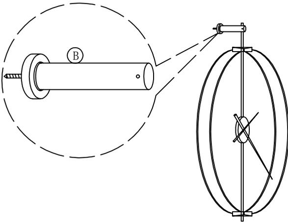
4. Bending the ring and assemble the outer ring of the clock.
