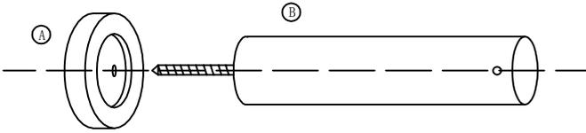
3. Be sure to tighten the fixed column B.
